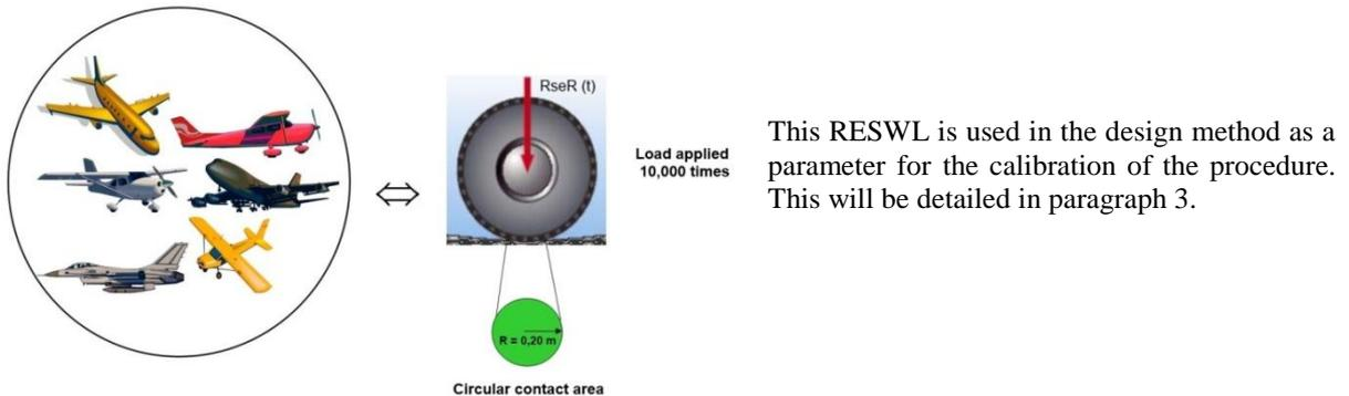
Figure 4: Definition of the rational equivalent single wheel load (RESWL)
