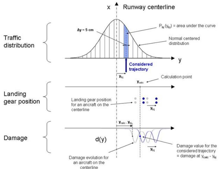
Figure 9: Consideration of lateral wandering for damage calculation
