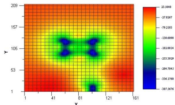
Figure 6: Example of fatigue tensile strain calculation for an A330-300 aircraft
