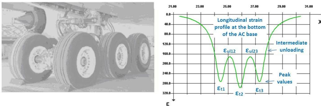
Figure 8: Illustration of the continuous integration of Miner's rule
