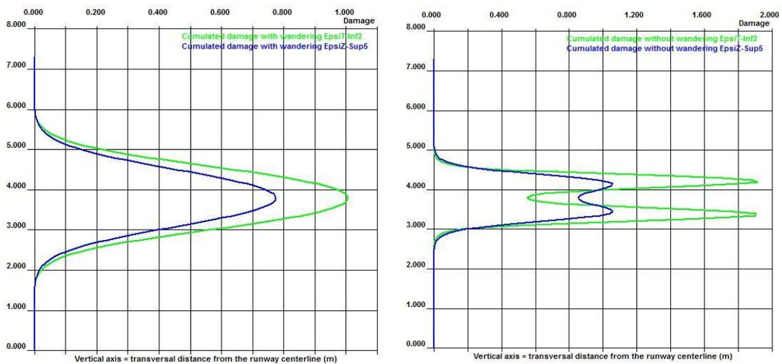
Figure 12: (a) Damage profile with wandering; (b) Damage profile without wandering
