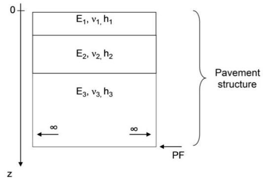
Figure 1: Description of the pavement structure
