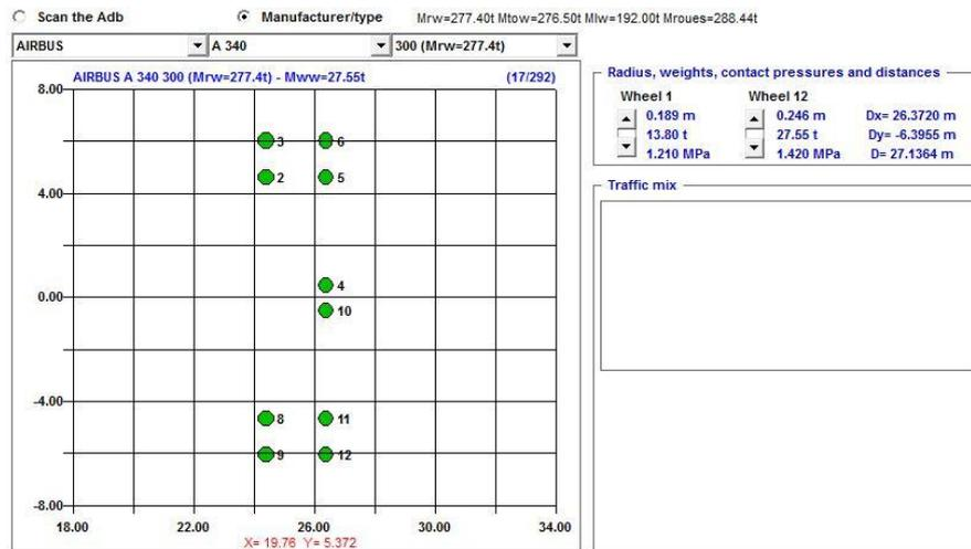
Figure 2: Description of landing gear loads
