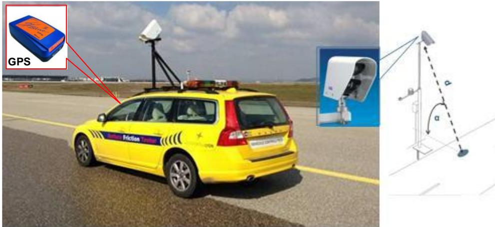
Figure 6: VAISALA sensors and its setting constraints
