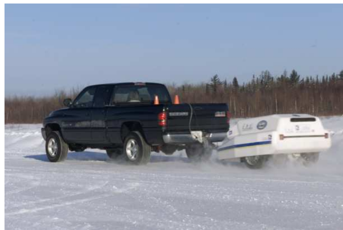
Continuous Friction Measuring Equipment \mu = F_h / F_v Eg: IMAG
