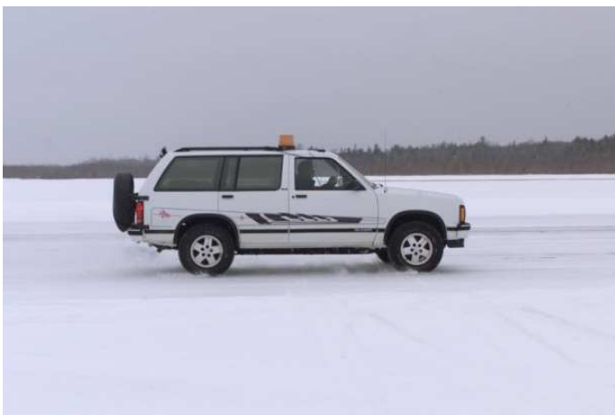
Decelerometer \mu = a/g CRFI
