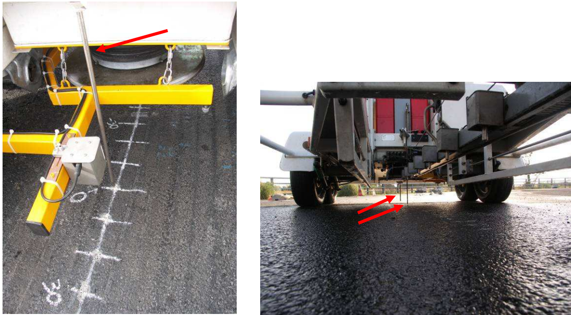
Fig. 3-3 Assisted positioning system over gages profiles (photographs by M. Broutin)
