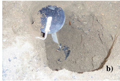
Figure 11 - a) Horizontal X and Y strain sensors (base of the asphalt layer), b) Vertical strain sensor (untreated materials), after [Broutin et al., 2008]
