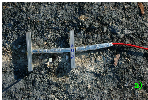
Figure 11 - a) Horizontal X and Y strain sensors (base of the asphalt layer), b) Vertical strain sensor (untreated materials), after [Broutin et al., 2008]
