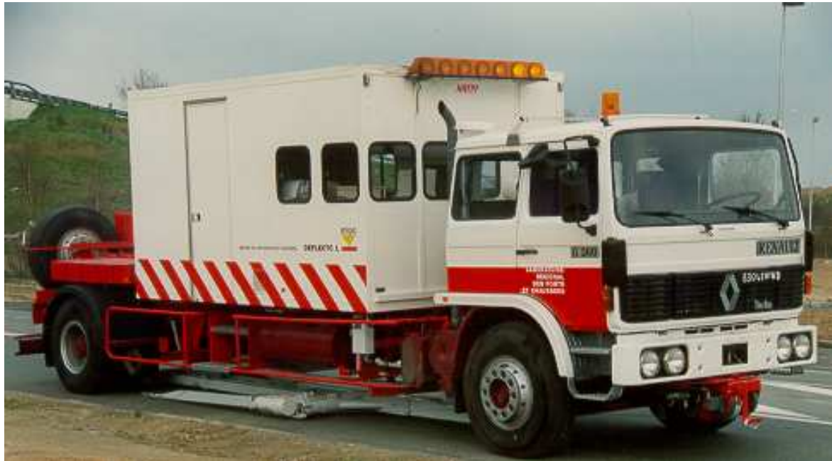
Fig. 0-15 The Lacroix Deflectograph (source: LCPC's database)
