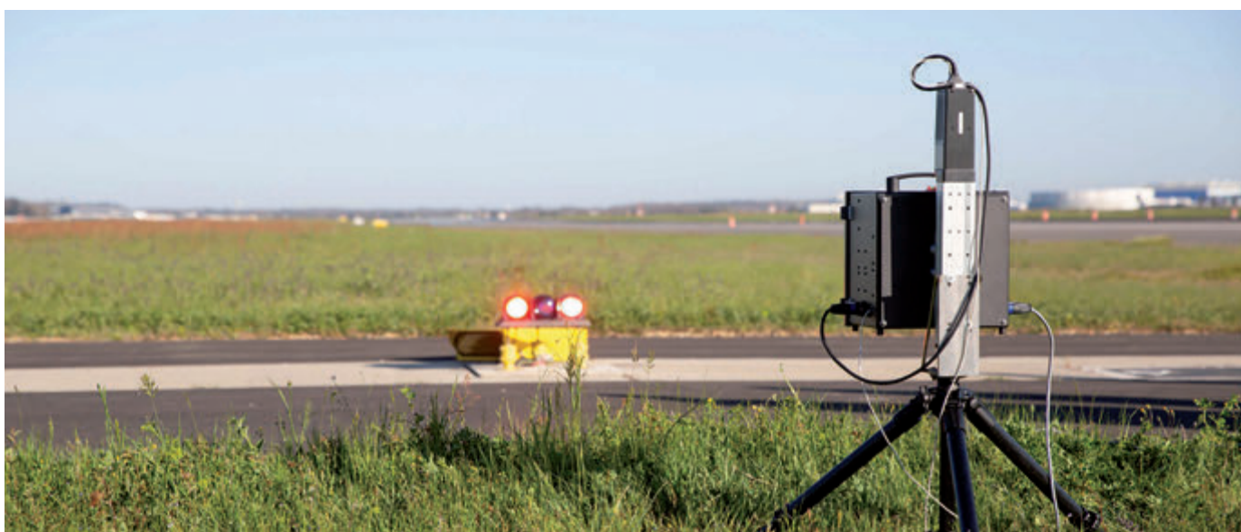
Figure 72: Measurement of the elevation setting angle of a PAPI light unit by the image analysis method at Toulouse Blagnac aerodrome.
