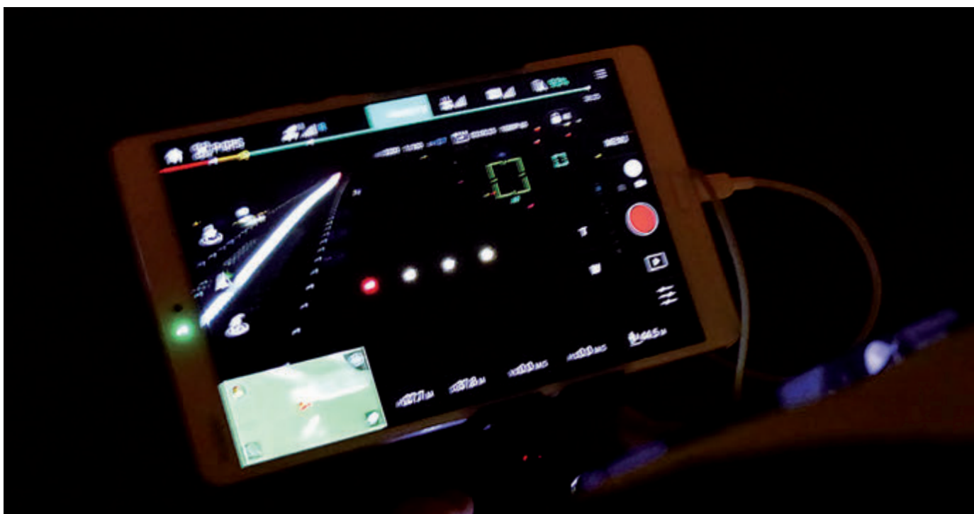
Figure 68: Real-time viewing of PAPI light units using a RPAS.
