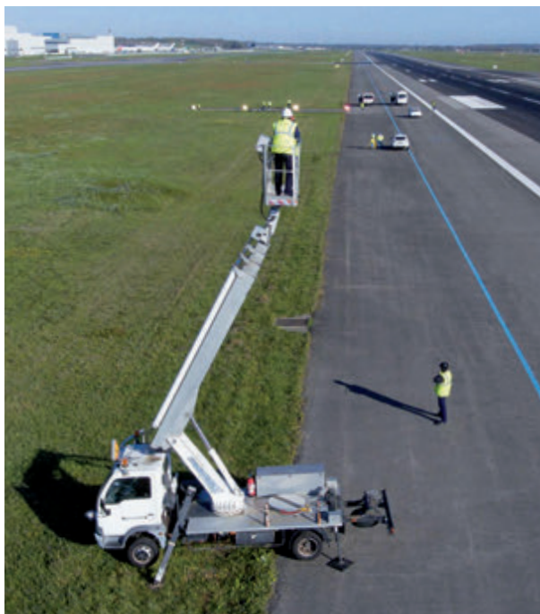
Figure 64: Lift platform positioned for the measurement of the elevation setting angle of a PAPI light unit at Toulouse Blagnac aerodrome.
