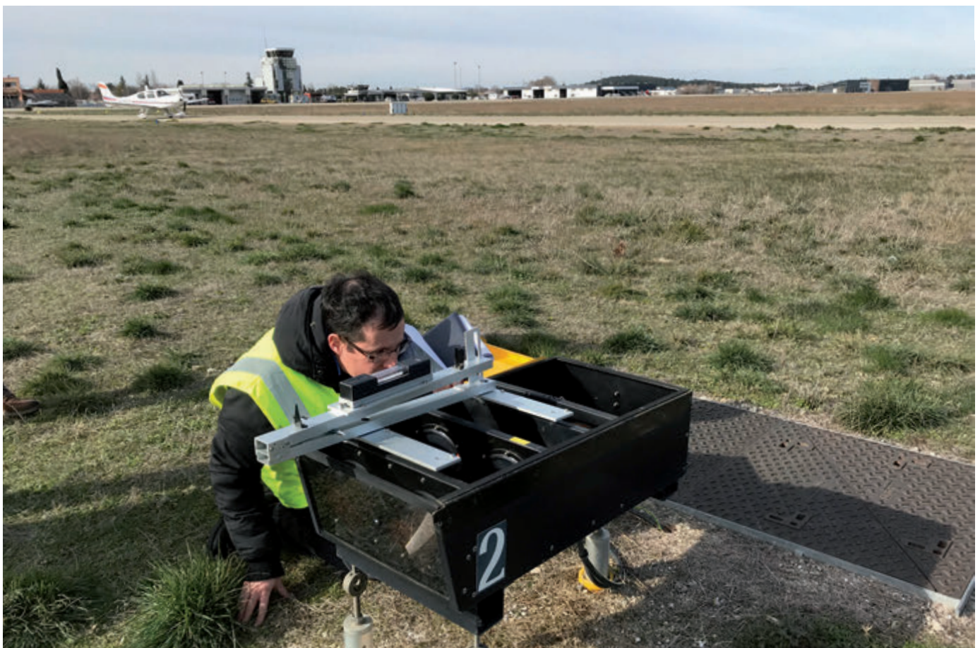
Figure 47: Checking of the elevation setting angle of the light units of a PAPI system at Avignon aerodrome.
