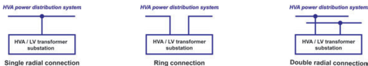
Figure 7: Possible types of connection of a HVA/LV transformer substation to a HVA power distribution system.
