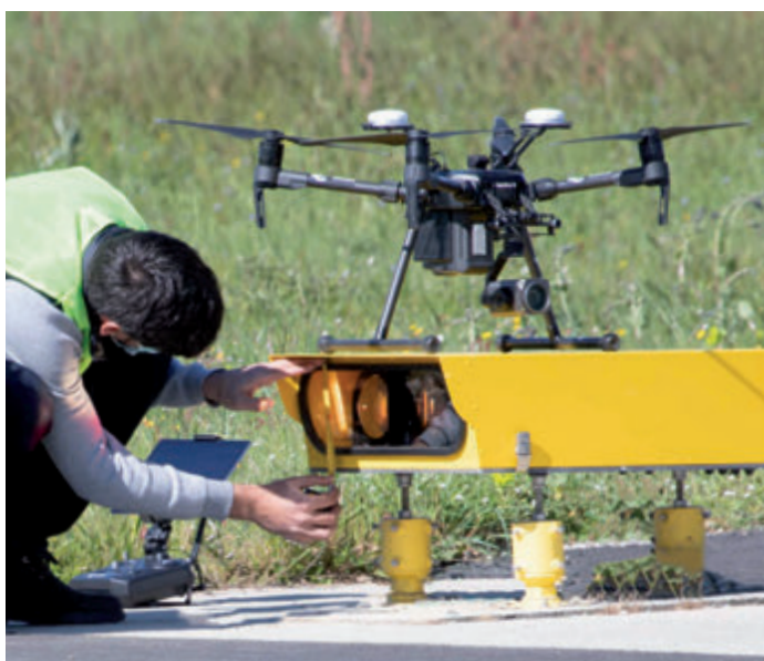
Figure 69: Consideration of the position of the GPS antenna of the RPA for the measurement of the elevation setting angle of a PAPI light unit by the RPAS method at Toulouse Blagnac aerodrome.
