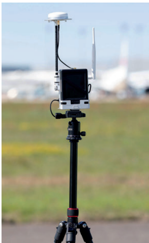
Figure 70: RTK base station located at the runway threshold for the measurement of the elevation setting angles of PAPI light units by the RPAS method at Toulouse Blagnac aerodrome.
