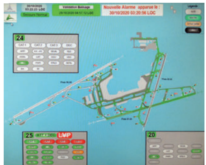
Figure 35: Control and command deck for the remote control of airfield lighting systems at Paris Orly aerodrome.
