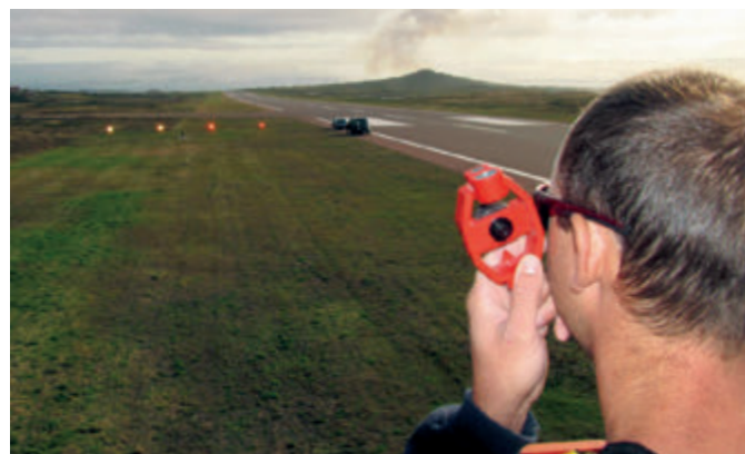
Figure 65: Observer on a lift platform, holding a targeting prism for the measurement of the elevation setting angle of a PAPI light unit.
