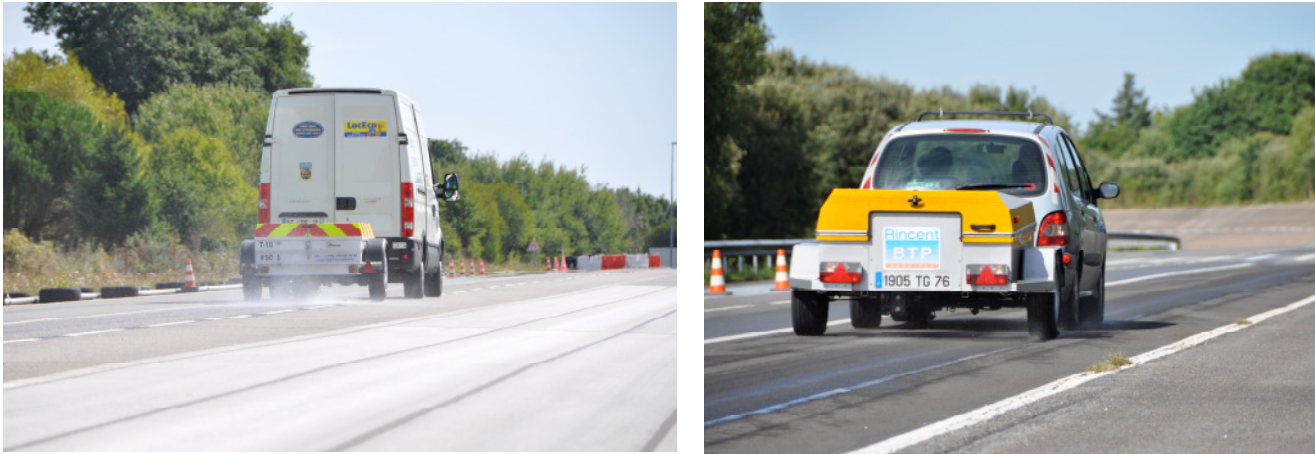
Figure 2: Pictures of different devices participating at certification campaign (type ASFT on left and type Sarsys STFT on right)
