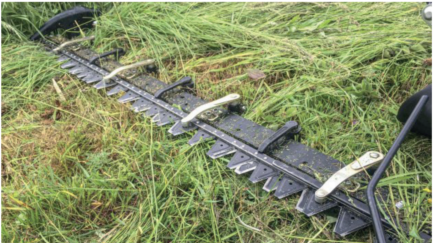
Figure 26 – Cutter bar with knives s 165/240.
