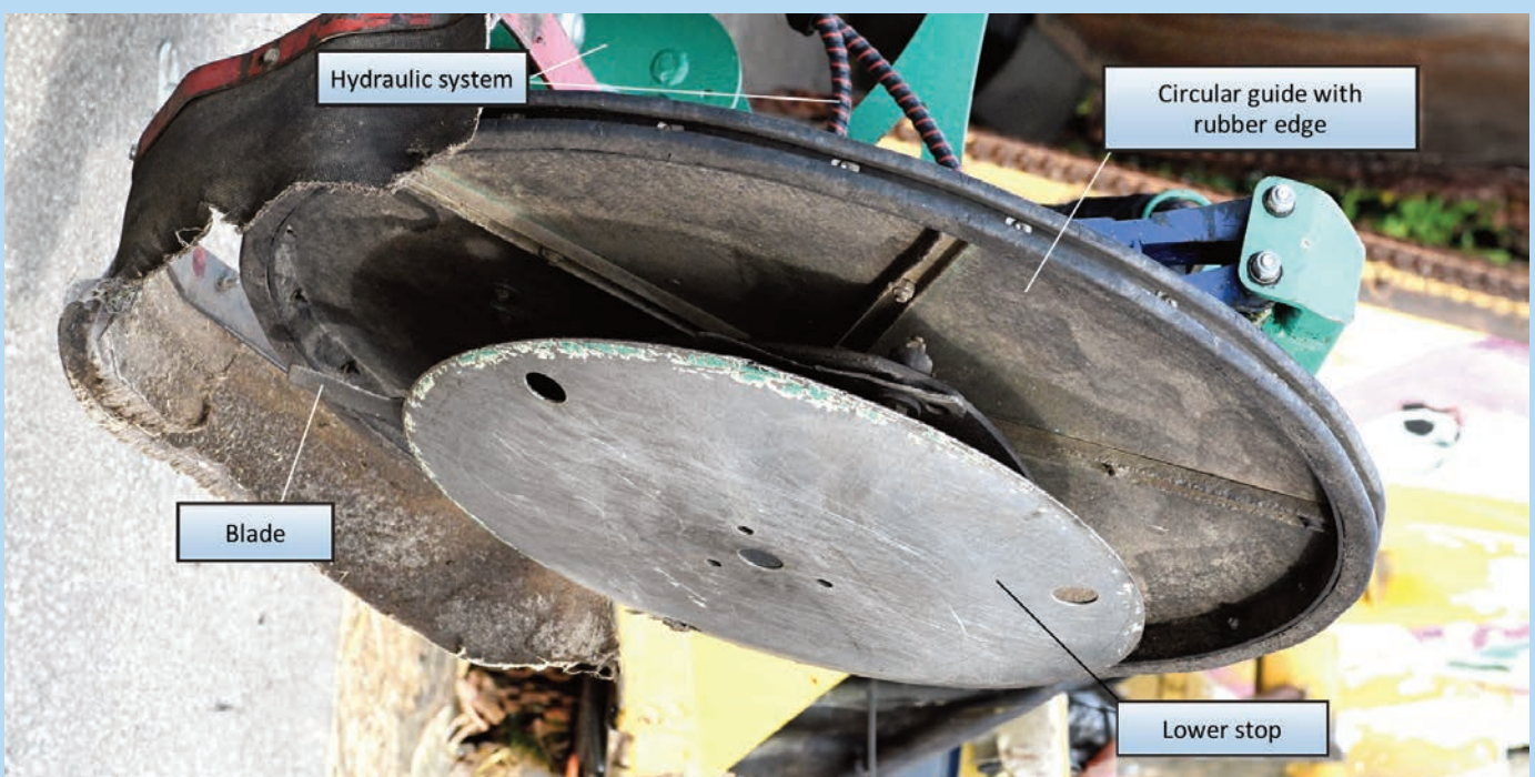
Figure 32 – Knife mower for fences, mounted on hydraulic cylinder.
