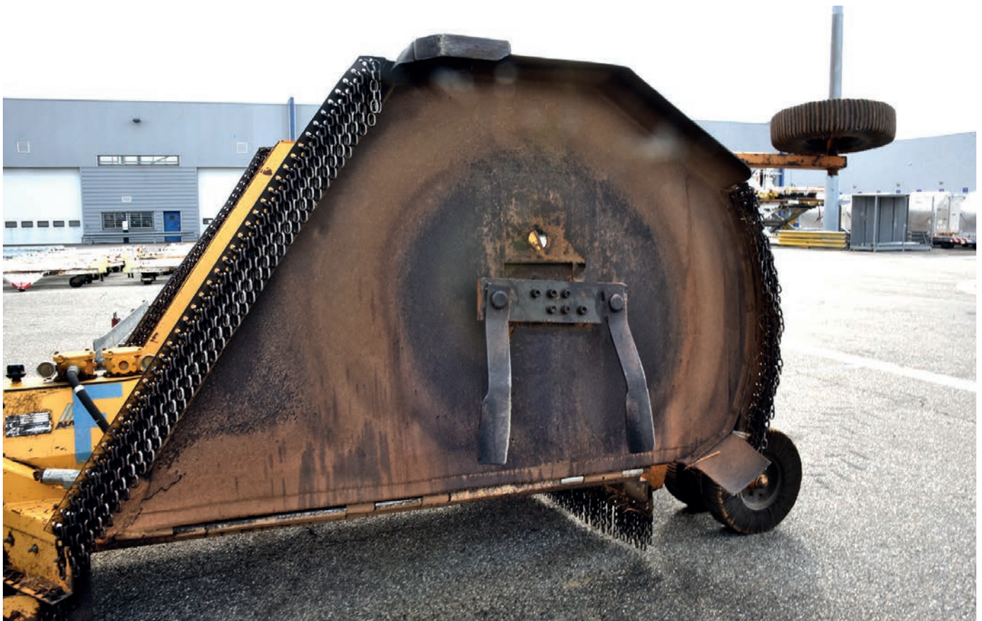
Figure 27 – 2-drum x 4-blade machine attachment, folded.
