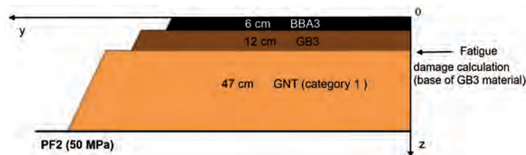
Figure 20: cross-section of the considered pavement structure
