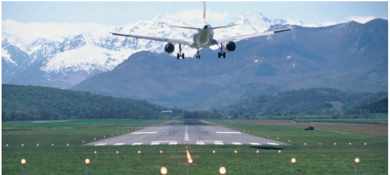
Figure 12: aircraft landing off-centre from the runway axis
