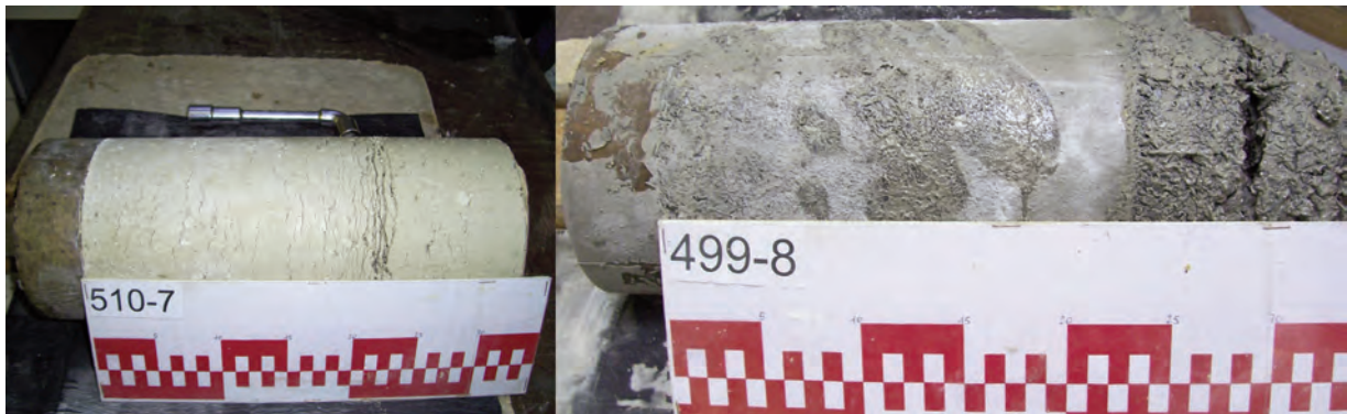
Figure 19: test samples after swell tests
