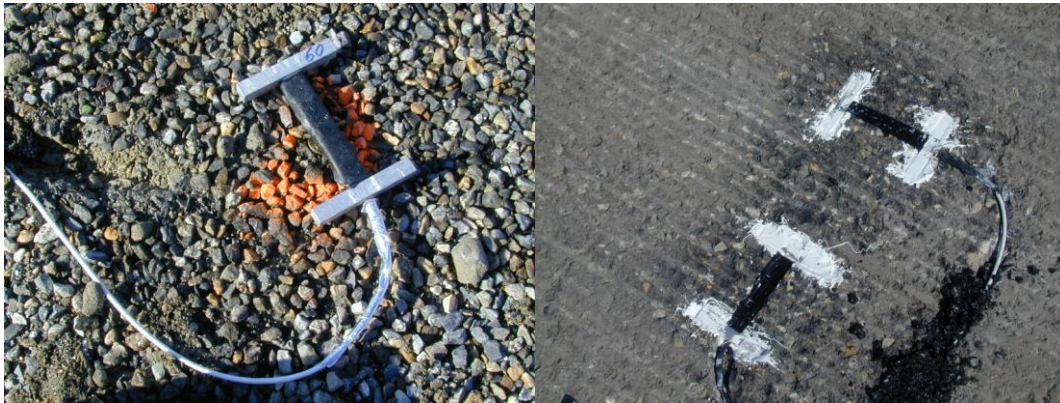
Figure 31: Horizontal strain gauges
