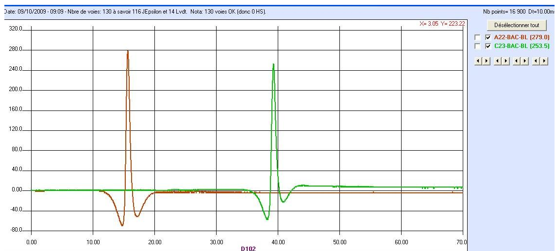
Figure 18: strains observed at bottom of base asphalt layer post reinforcement
