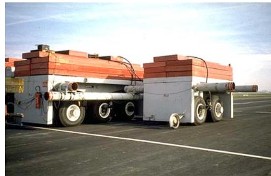
A reference module (as twin) had to be passed on flexible pavement before every simulator configuration, for the instrumentation calibration. (cf. § II-2-3)
