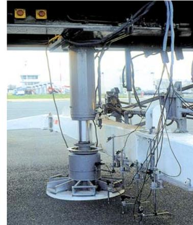
Vertical deformations are measured by gauges (one through the plate, and the others at regular distances from the edge of the plate) in order to define the shape of the deflection curve.
