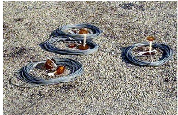
Vertical strain sensors on top subgrade and their cabling.
