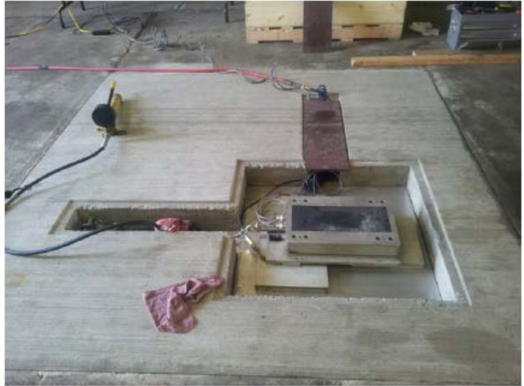
Figure 12. Force Calibration Pit and Platform
