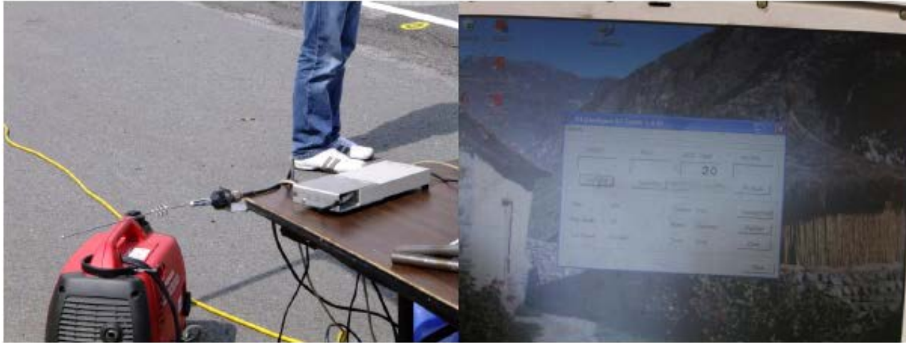
Figure 17. STALKER radar system and display used for speed calibration station.
