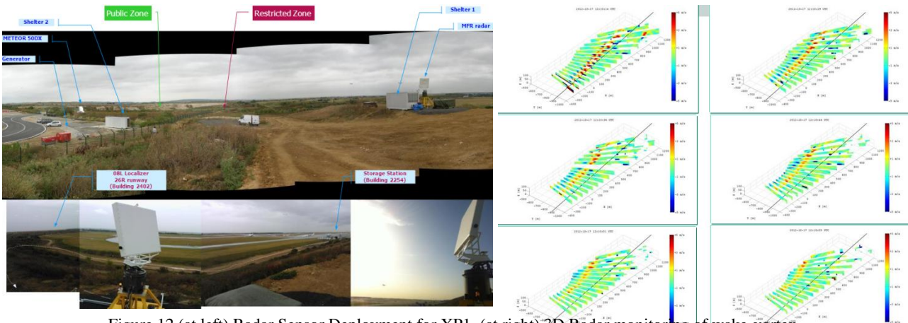
Figure 12.(at left) Radar Sensor Deployment for XP1, (at right) 3D Radar monitoring of wake-vortex
