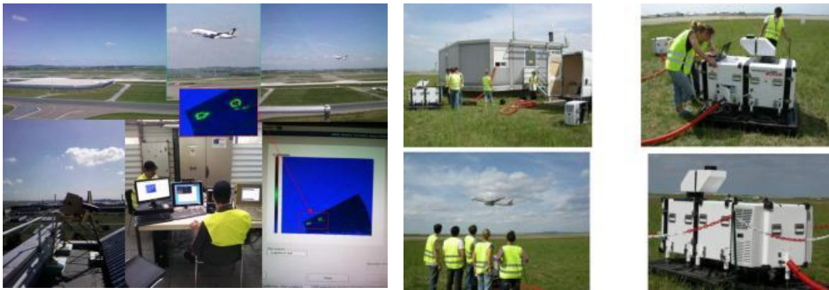
Figure 9. (at left) Thales Wake-Vortex Radar Sensor, (at right) Leosphere Wake-Vortex Lidar Sensor
